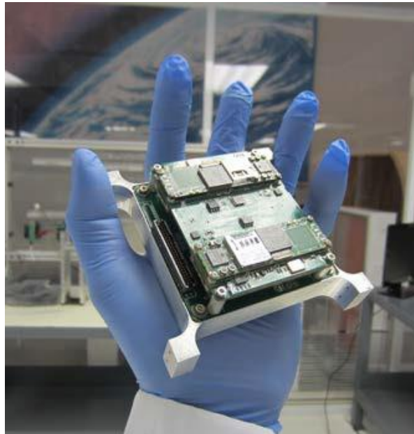
Figure 2 - DM Flight Prototype – Integrated Payload Processor Subsystem
